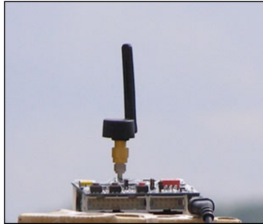
Figure 2. Receiver module with external antenna mounted on top of tripod
